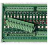
Easily exchangeable connections and easily replaceable terminal blocks.
